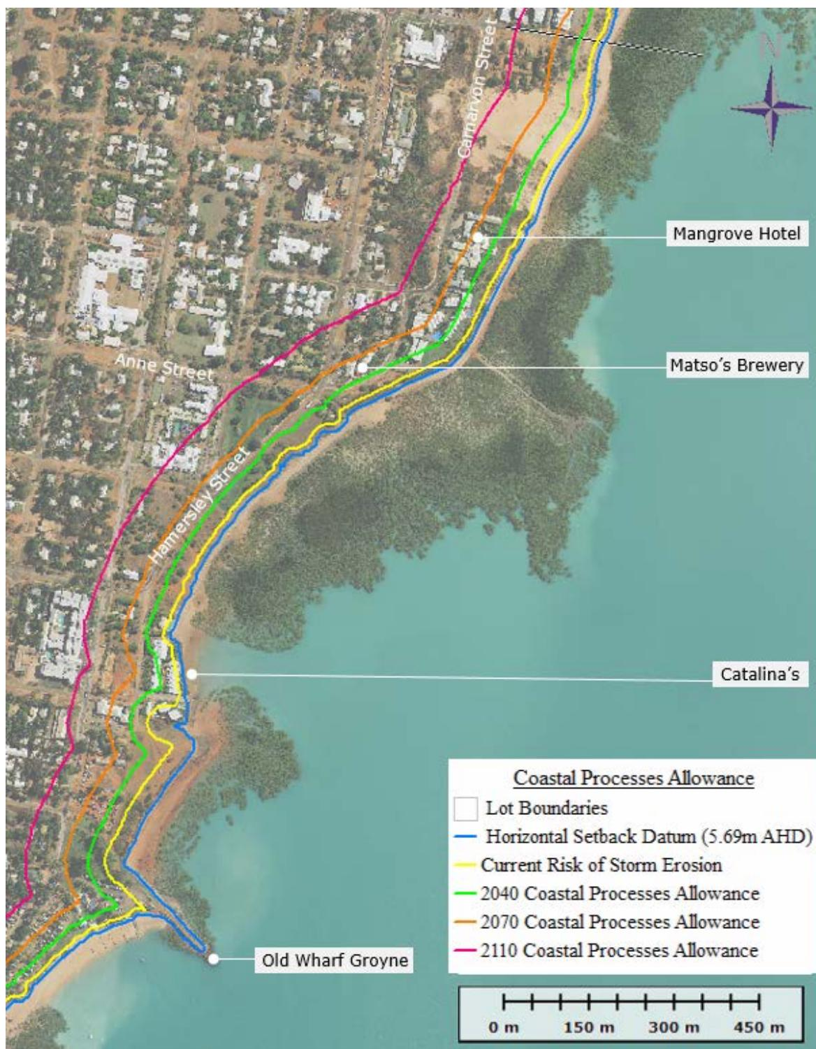
Figure 4.13: Town Beach Compartment showing coastal processes erosion allowances recommended for future planning periods north of the old jetty area
