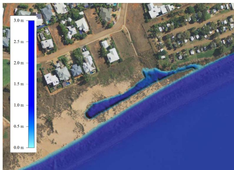
**Figure 6.11: Low Point in dune adjacent Demco Drive showing potential inundation in the ARI100yr water level ('bathtub' mapping approach based on LiDAR).**
