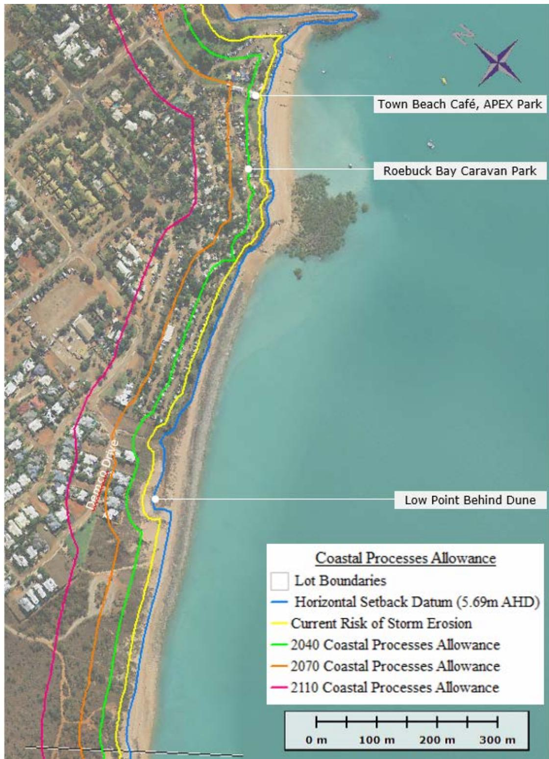
**Figure 4.12: Town Beach Compartment showing coastal processes erosion allowances recommended for future planning periods south of the old jetty area**
