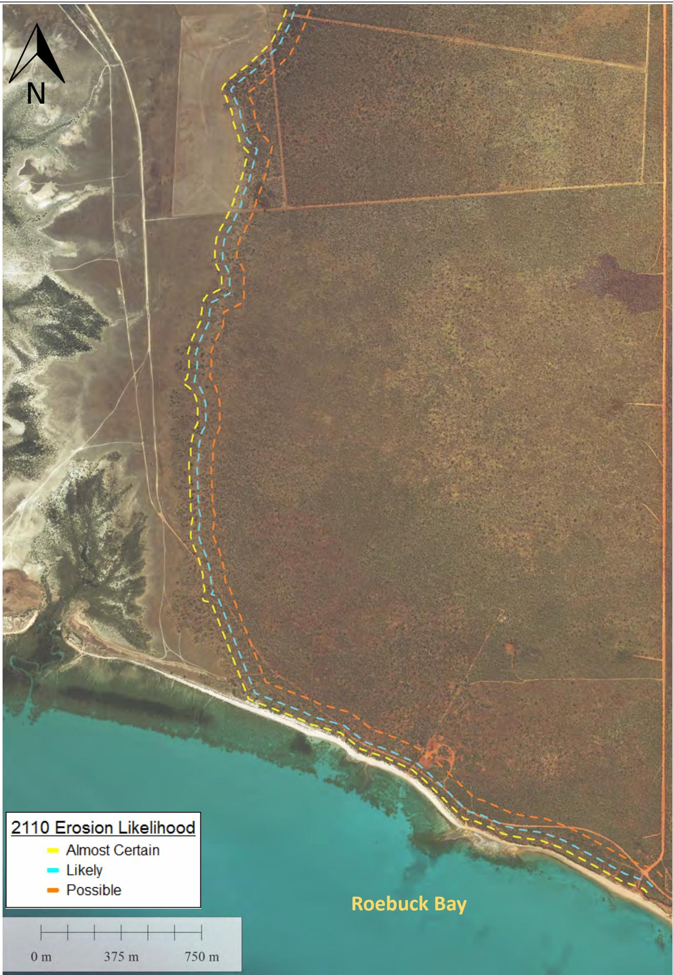
Figure B9.3 Coastal Compartment 9 Dampier Ck East: Storm Tide Erosion Likelihood 2110
