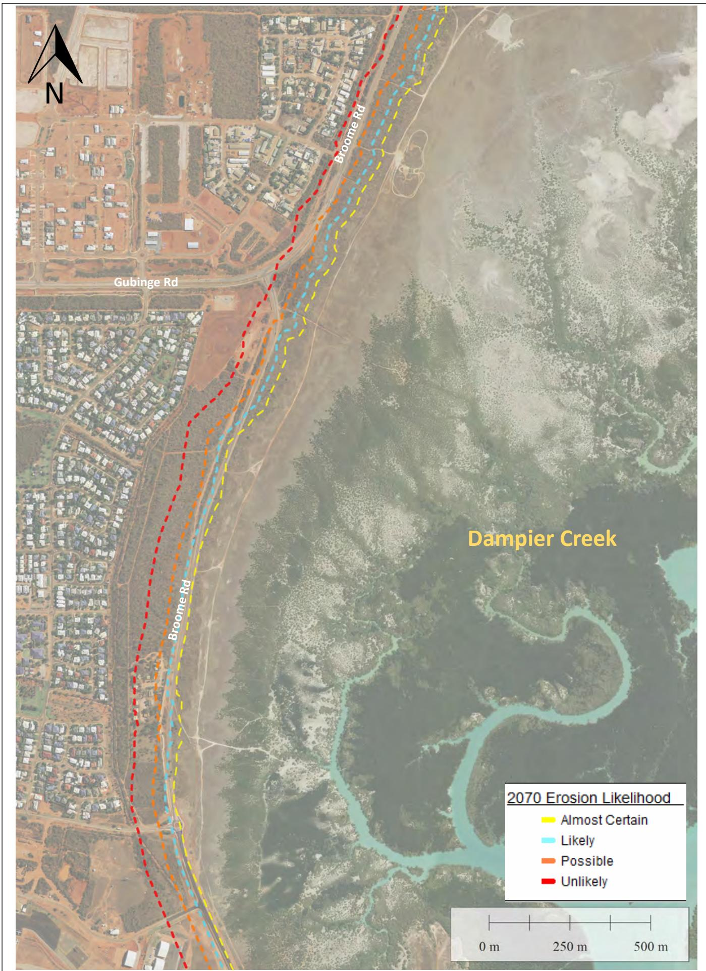
Figure B8.2 Coastal Compartment 8 Dampier Ck Inner: Storm Tide Erosion Likelihood 2070
