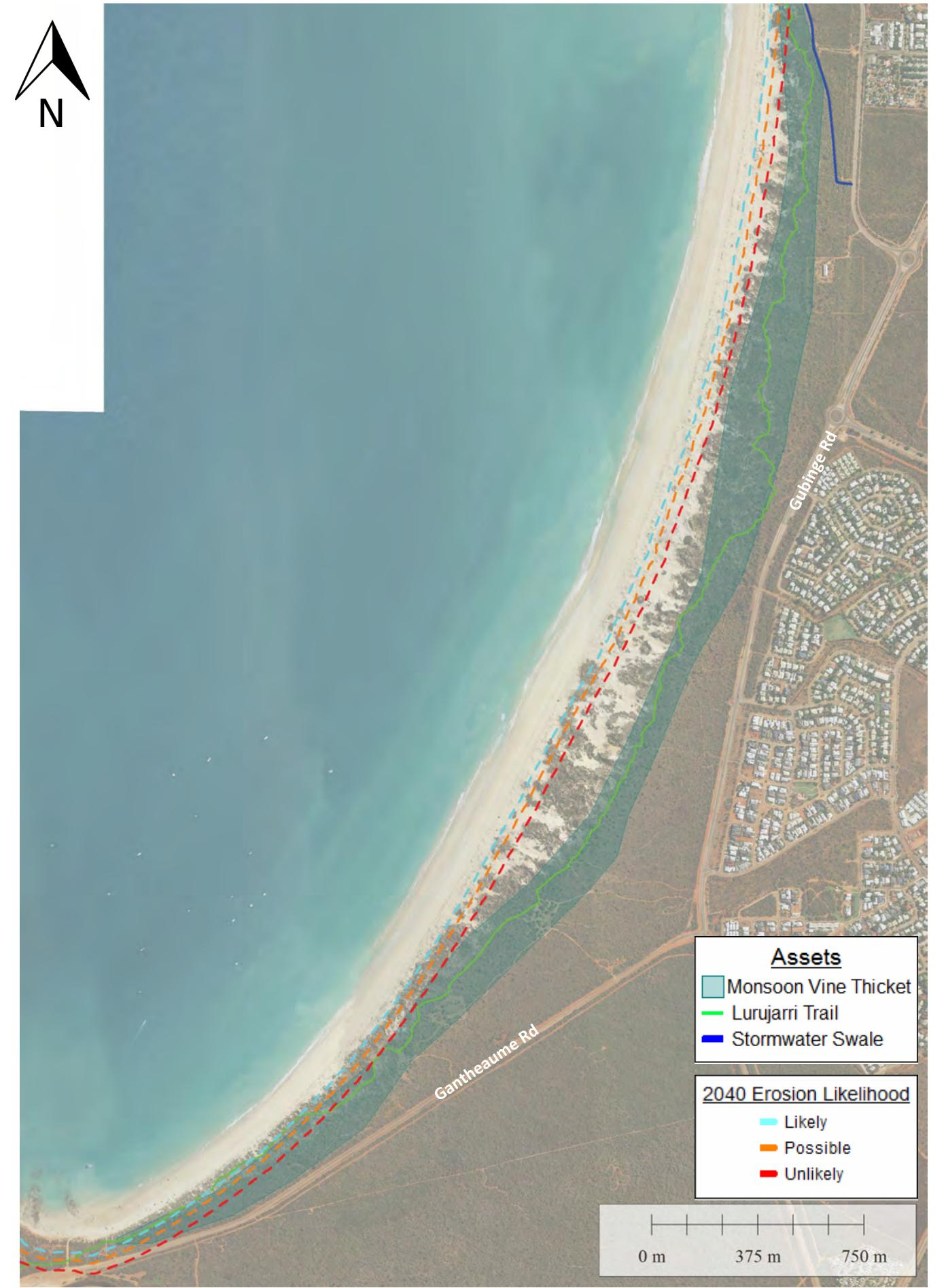
Figure B1.7 Coastal Compartment 1 Cable Beach South: Erosion Likelihood 2040
