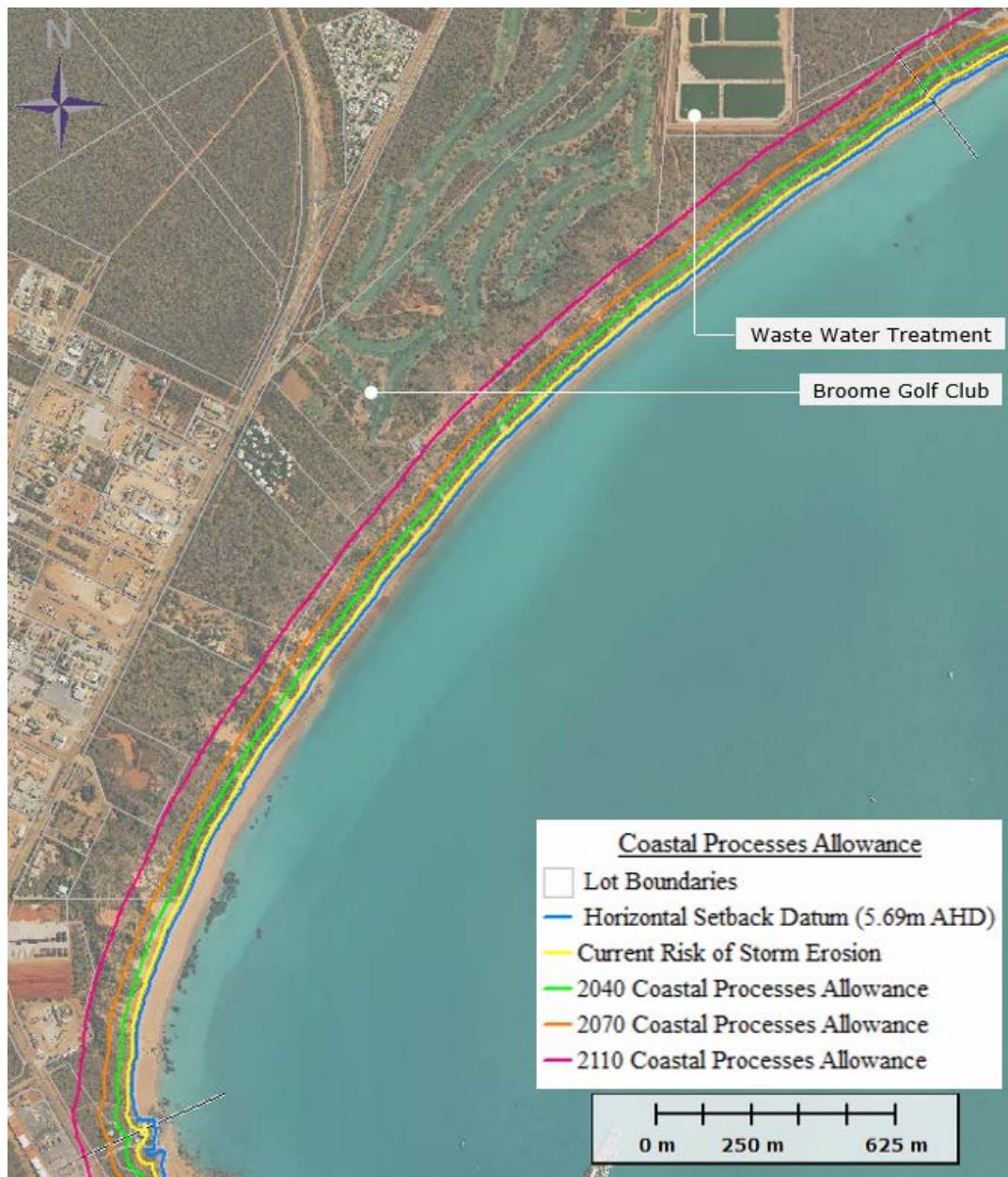
**Figure 4.10: Simpsons Beach Compartment showing coastal processes erosion allowances recommended for future planning periods**
