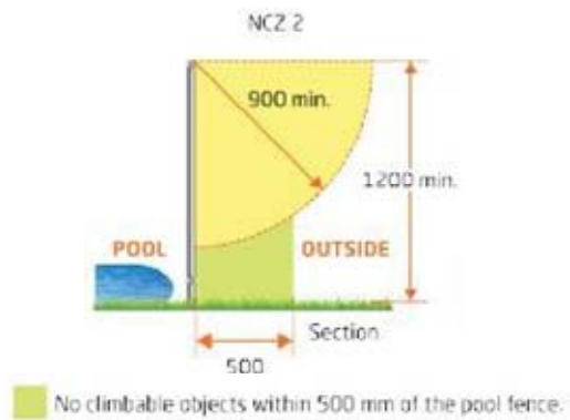
900mm non-climbable zone from top of barrier outside Nothing within 500mm of the outside of the barrier
