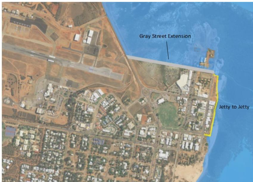
**Figure 6.23: Concept Option 2 proposing Gray Street Extension as coastal protection structure across northern side and seawall/walkway on eastern side of Chinatown.**
