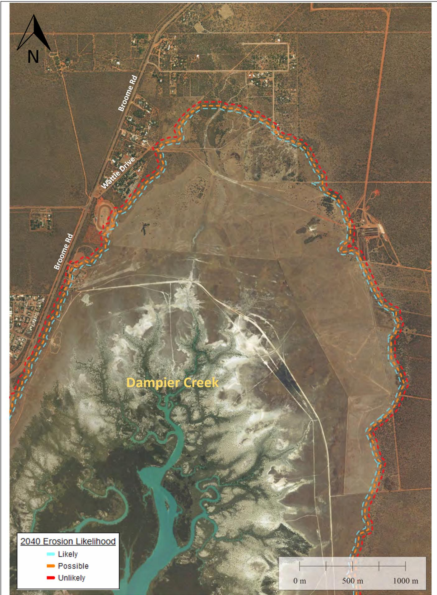
Figure B8.4 Coastal Compartment 8 Dampier Ck Inner: Storm Tide Erosion Likelihood 2040
