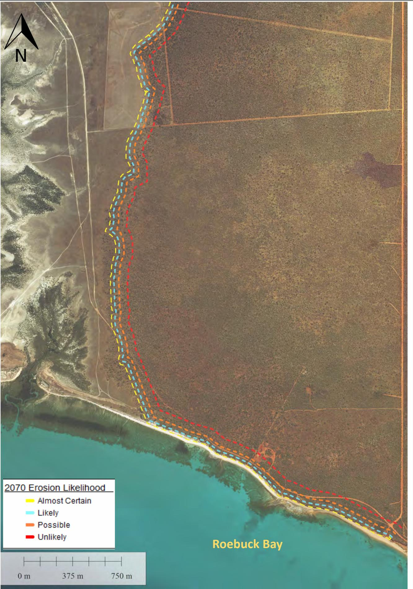
Figure B9.2 Coastal Compartment 9 Dampier Ck East: Storm Tide Erosion Likelihood 2070
