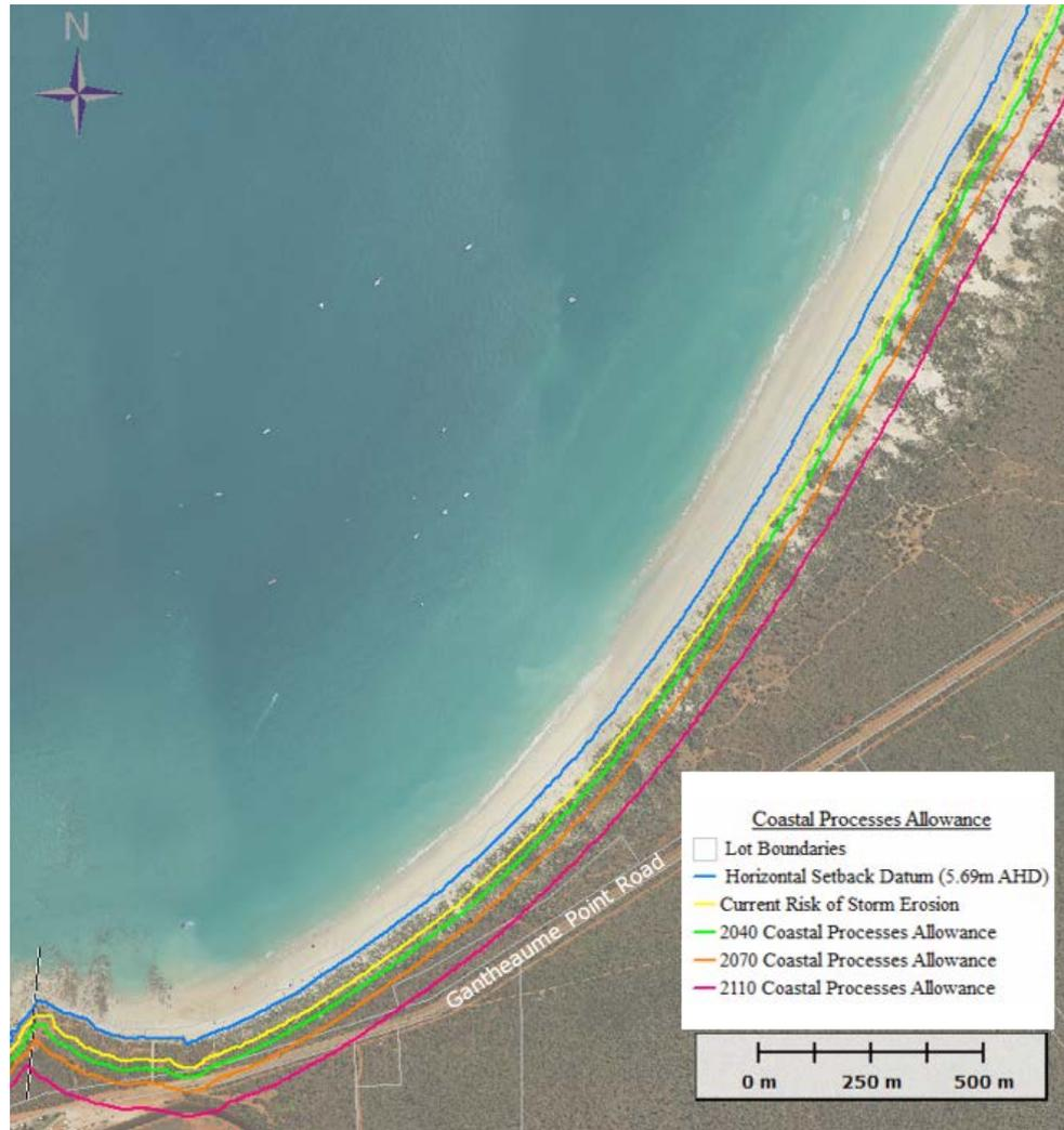
**Figure 4.5: Cable Beach Coastal Compartment (South, lower) showing coastal processes erosion allowances recommended for future planning periods**
