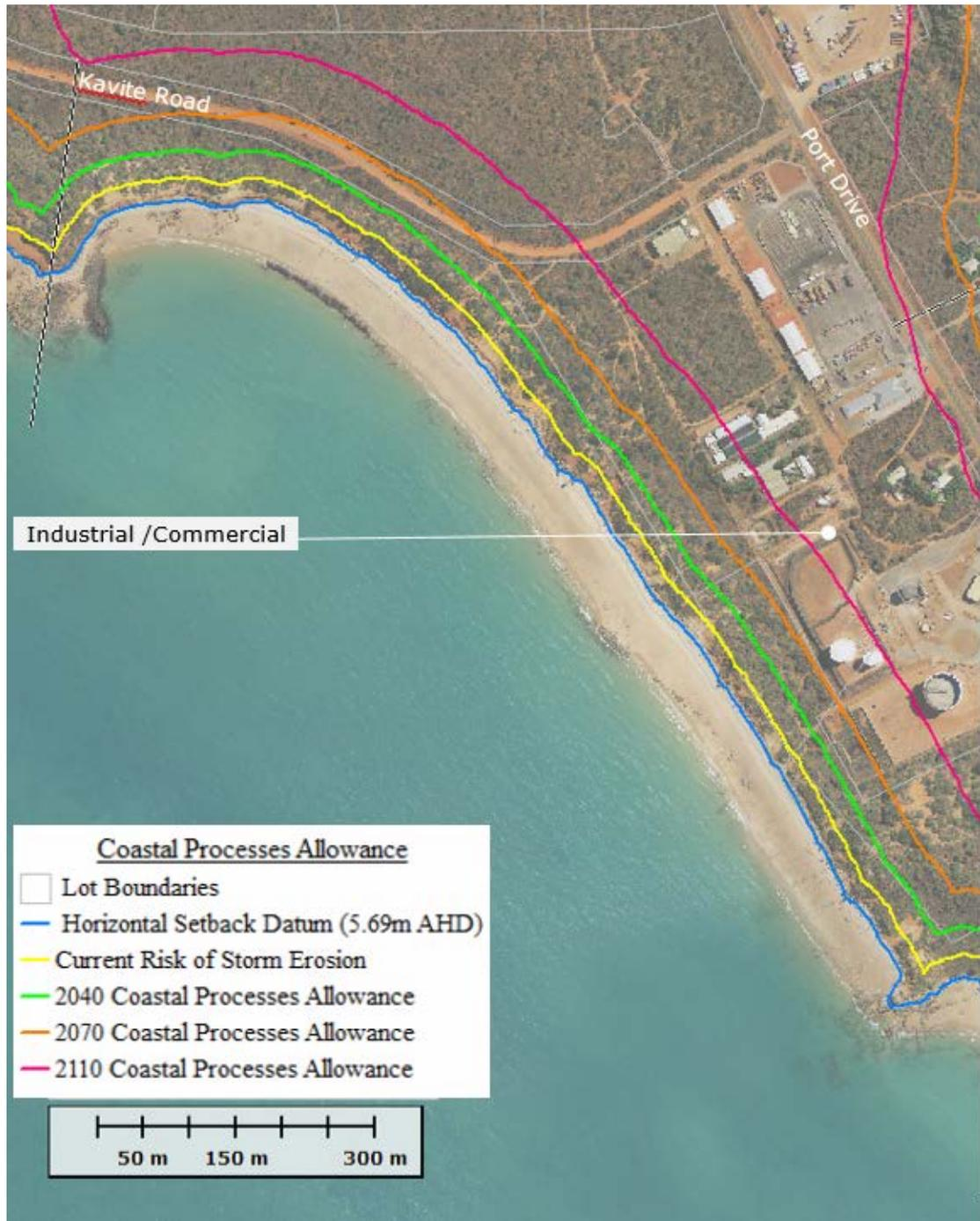
Figure 4.8: Entrance Point Compartment (west side) showing coastal processes erosion allowances recommended for future planning periods
