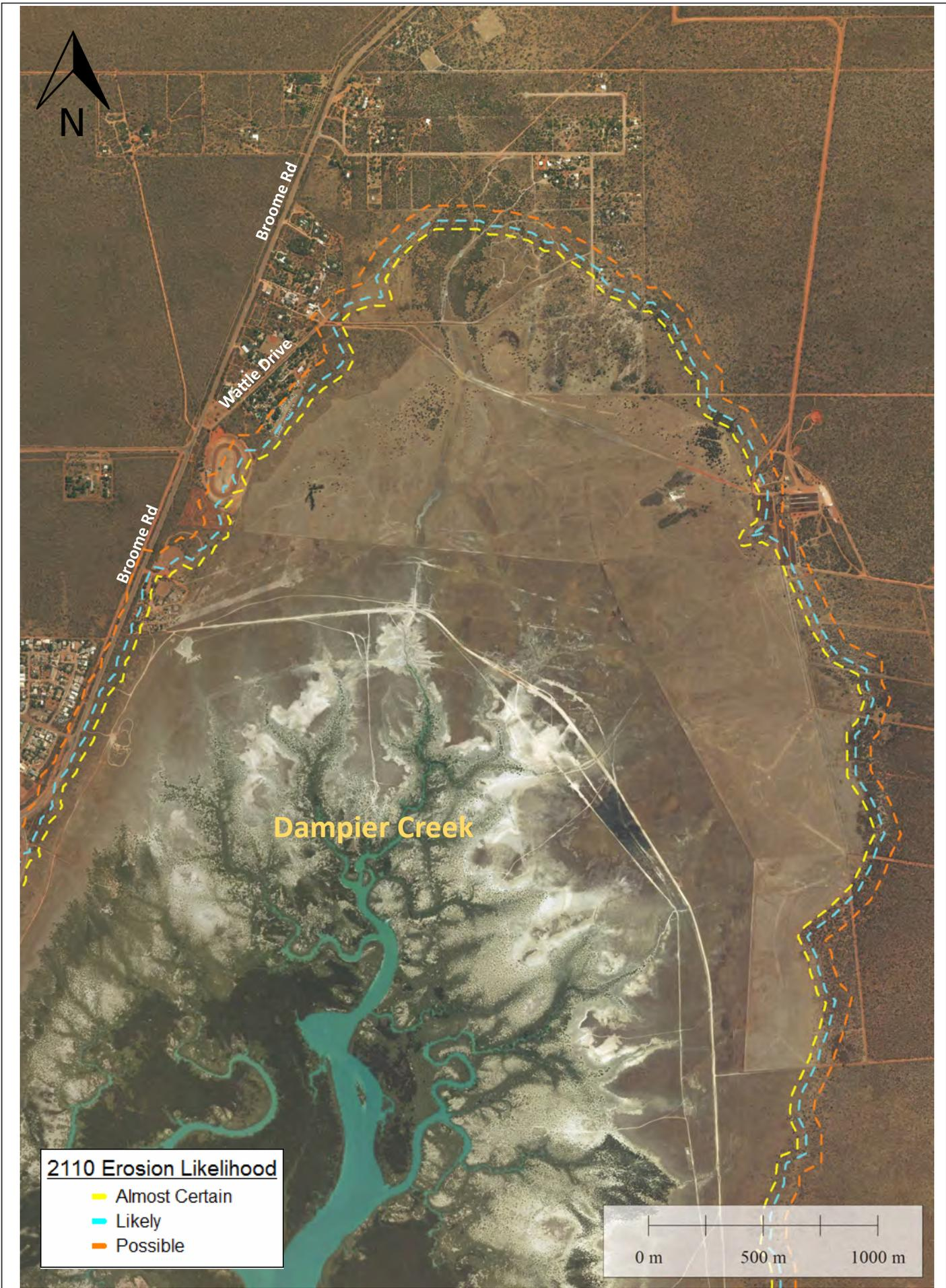
Figure B8.6 Coastal Compartment 8 Dampier Ck Inner: Storm Tide Erosion Likelihood 2110
