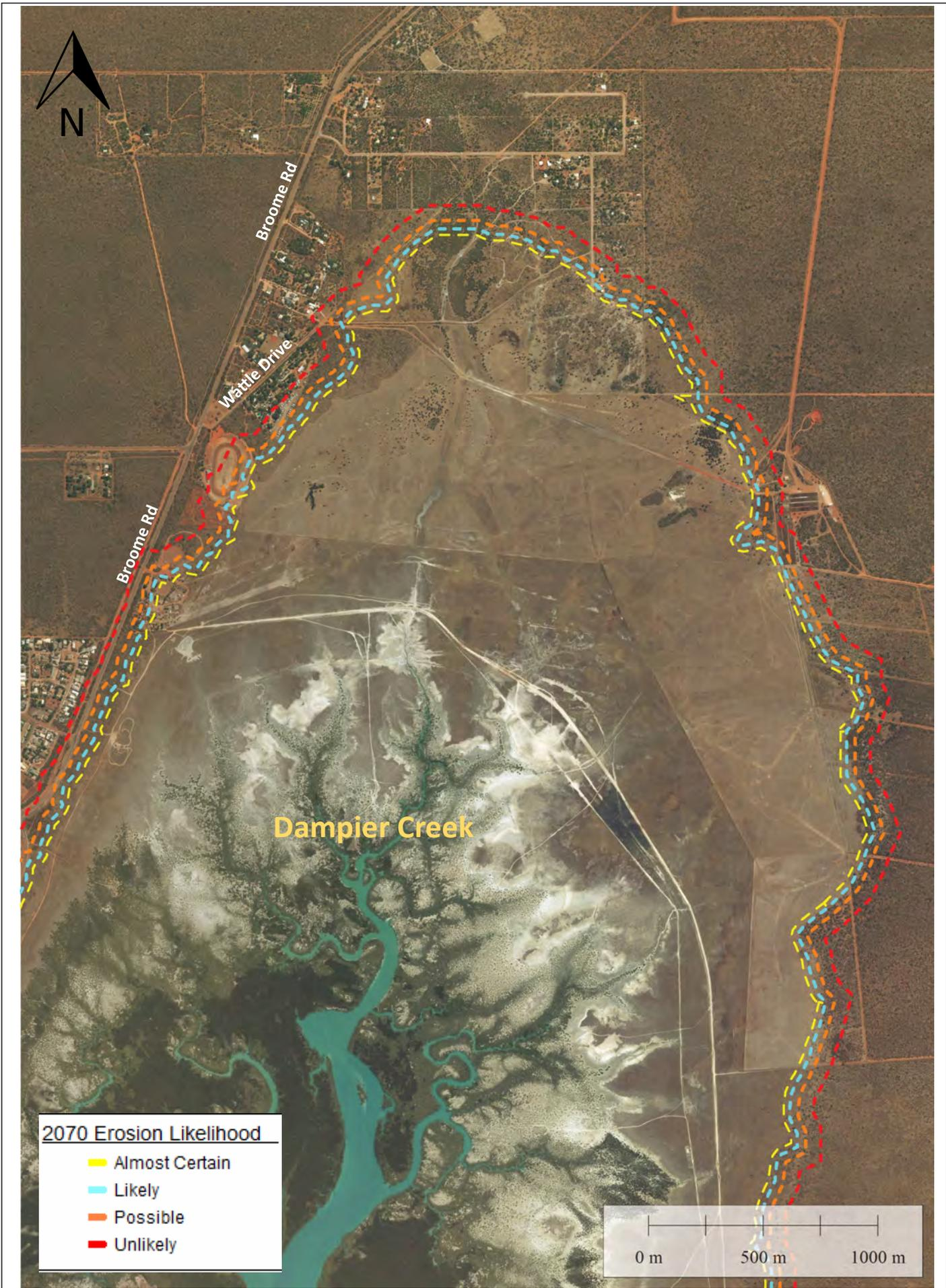
Figure B8.5 Coastal Compartment 8 Dampier Ck Inner: Storm Tide Erosion Likelihood 2070
