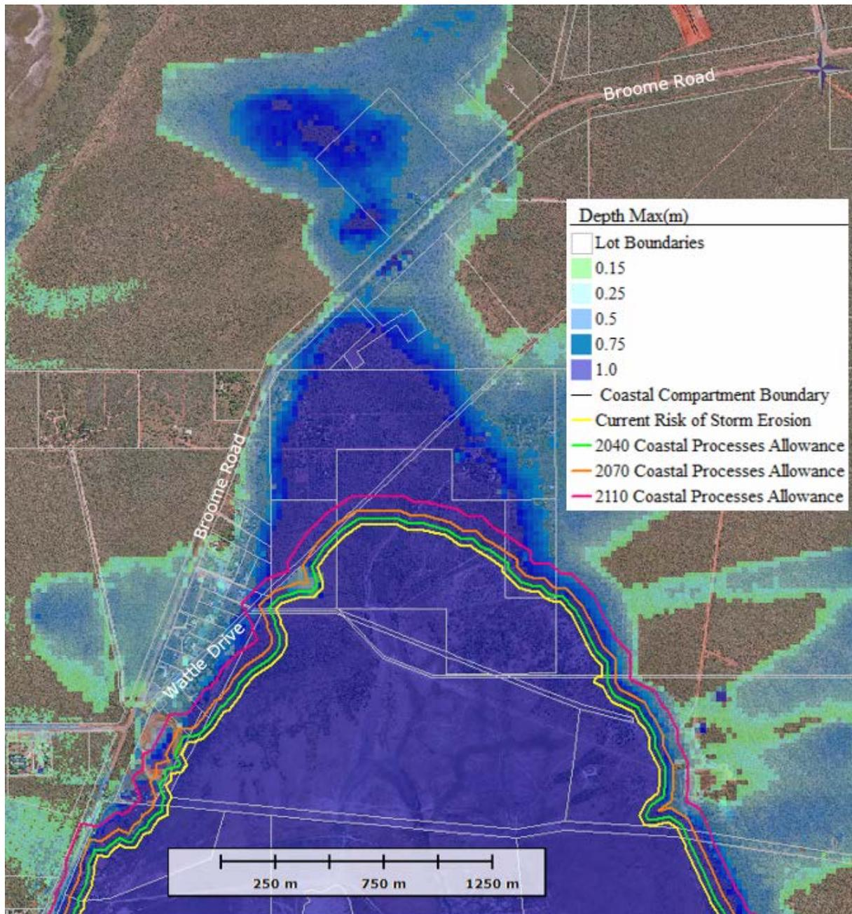
**Figure 4.19: Dampier Creek Inner Compartment (upper) showing coastal processes erosion allowances recommended for future planning periods, and inundation extents for the 2110 500-yr ARI event.**
