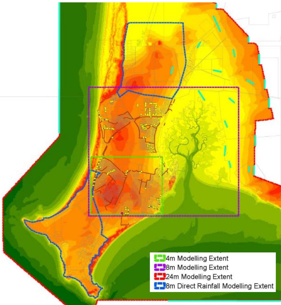
Figure 3.2: Numerical model grid size through the town site study area (Cardno 2015)
