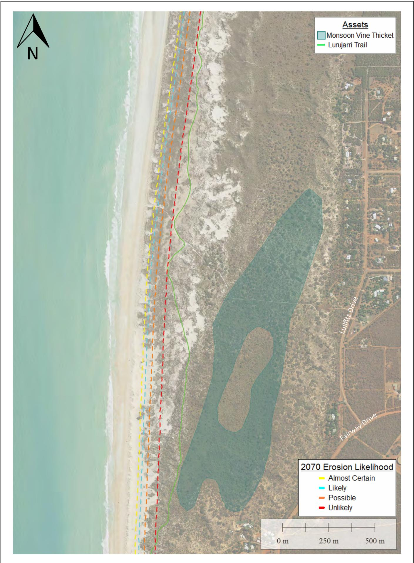
Figure B1.2 Coastal Compartment 1 Cable Beach North : Erosion Likelihood 2070
