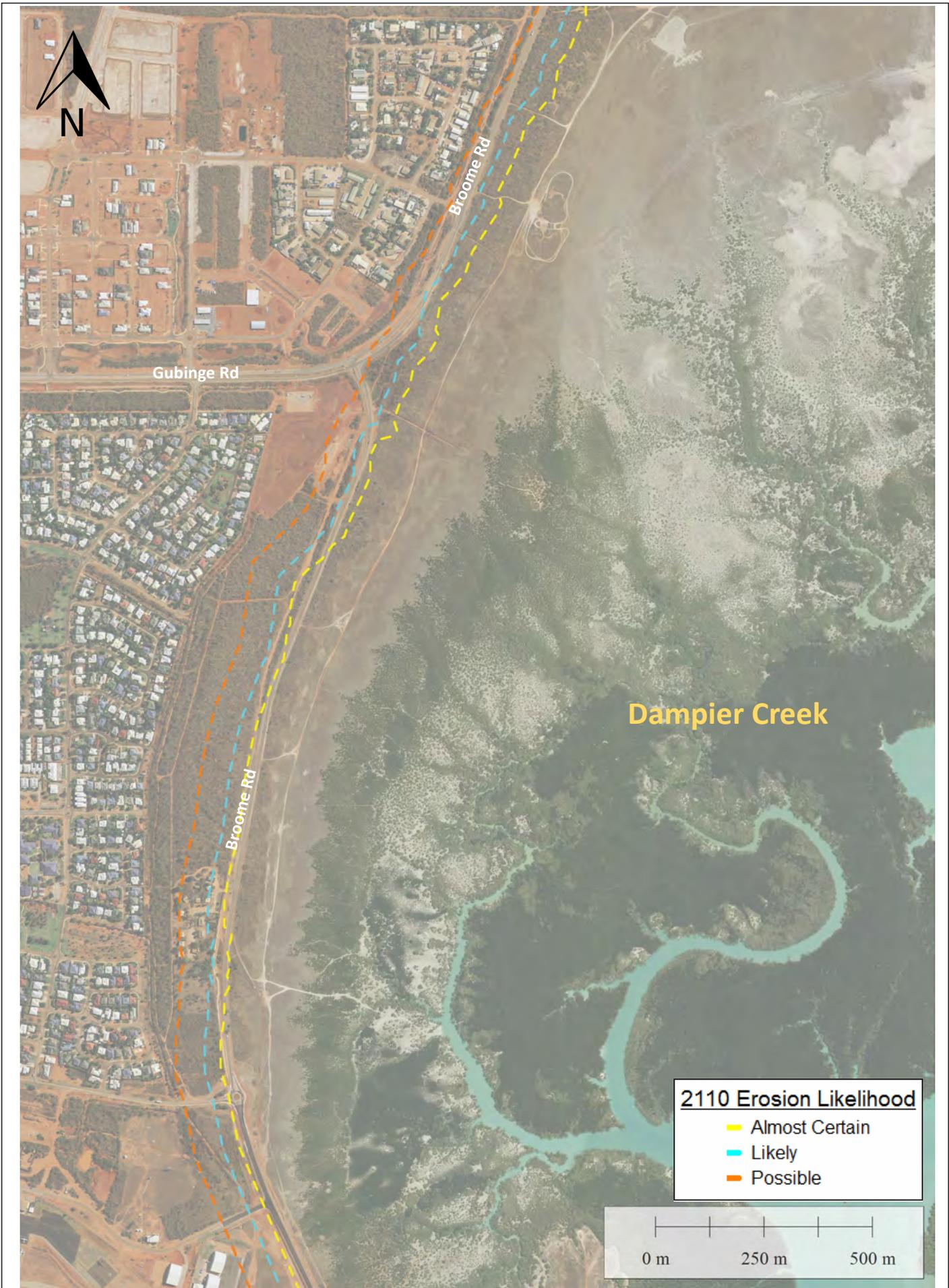
Figure B8.3 Coastal Compartment 8 Dampier Ck Inner: Storm Tide Erosion Likelihood 2110
