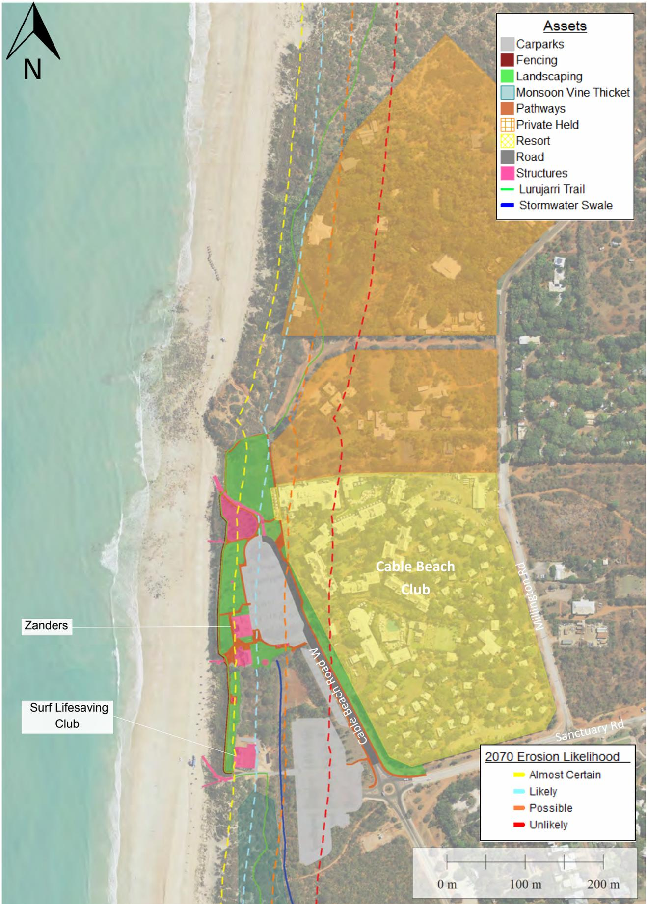
Figure B1.5 Coastal Compartment 1 Cable Beach Central: Erosion Likelihood 2070
