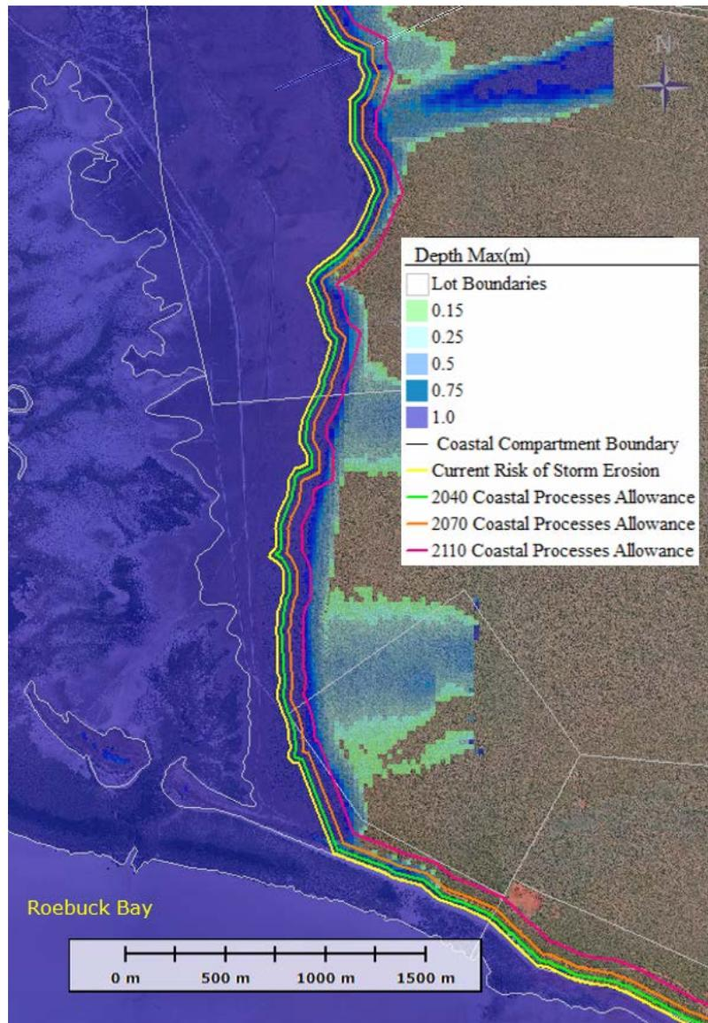
Figure 4.20: Dampier Creek East Compartment showing coastal processes erosion allowances recommended for future planning periods, and inundation extents for the 2110 500-yr ARI event
