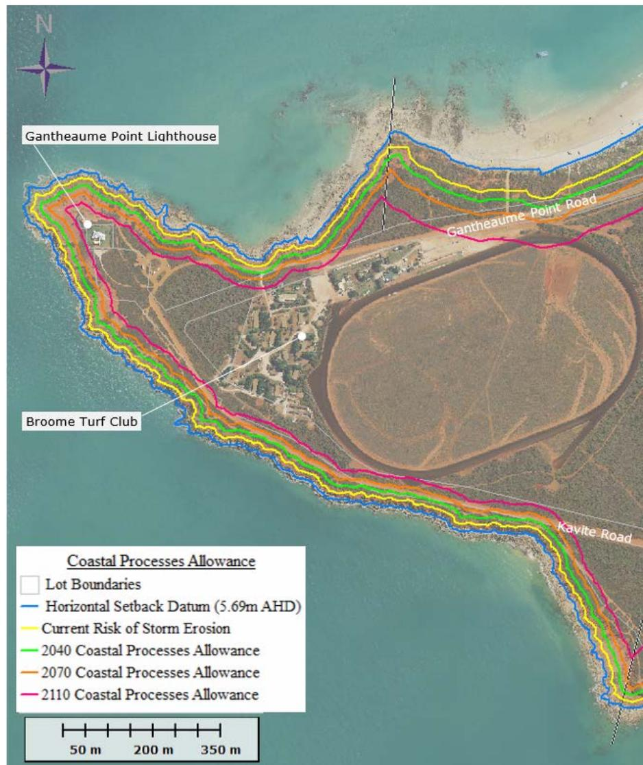
Figure 4.6: Gantheaume Cliffs Compartment showing coastal processes erosion allowances recommended for future planning periods
