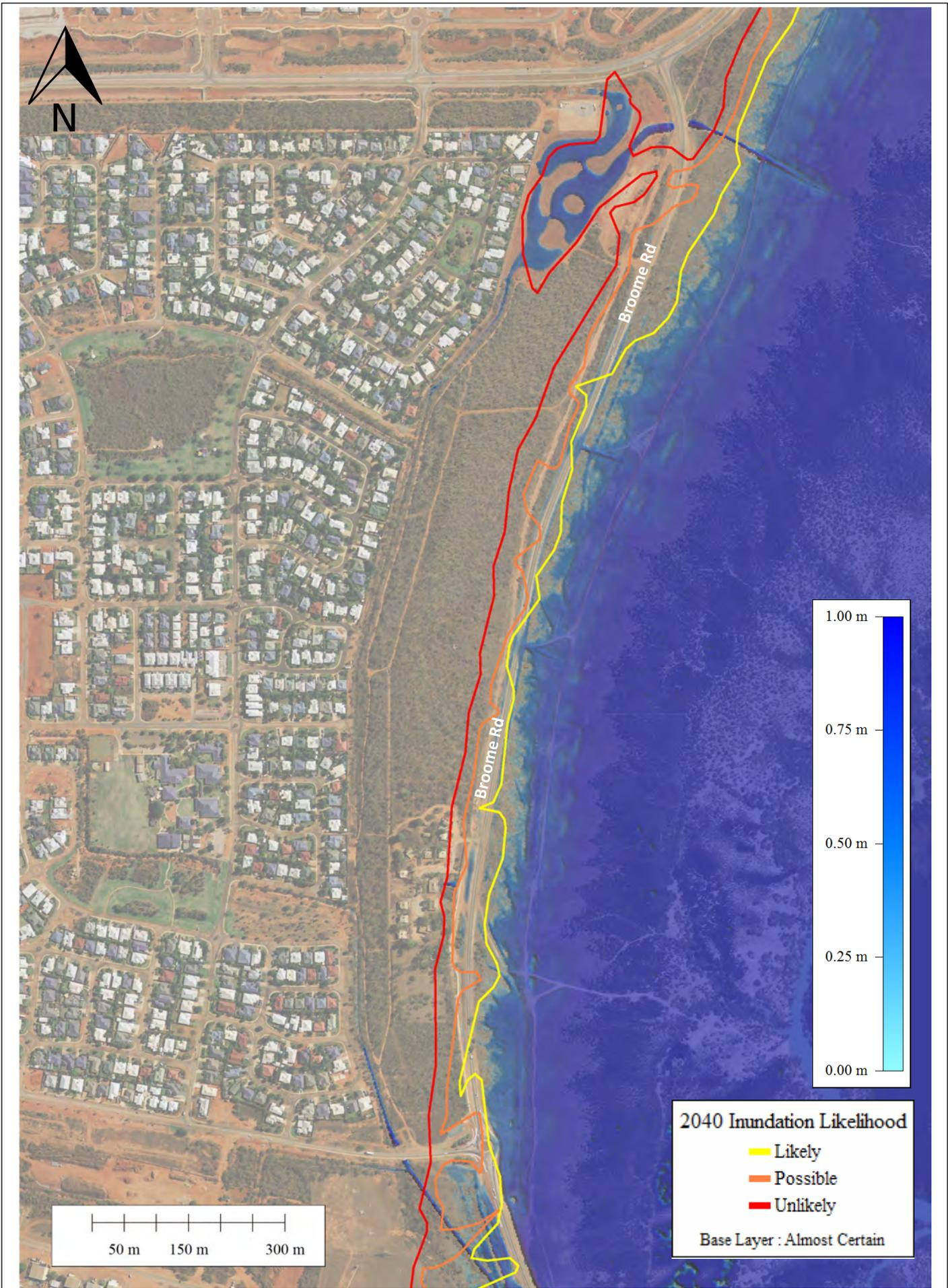
Figure B8.7 Coastal Compartment 8 Dampier Ck Inner: Storm Tide Inundation Likelihood 2040
