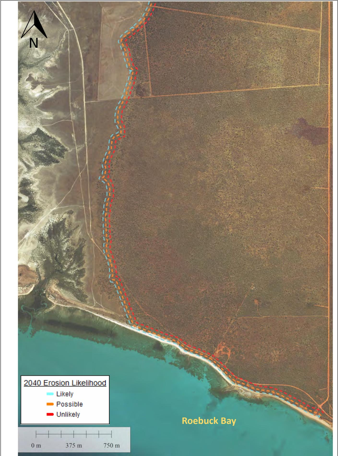
Figure B9.1 Coastal Compartment 9 Dampier Ck East: Storm Tide Erosion Likelihood 2040
