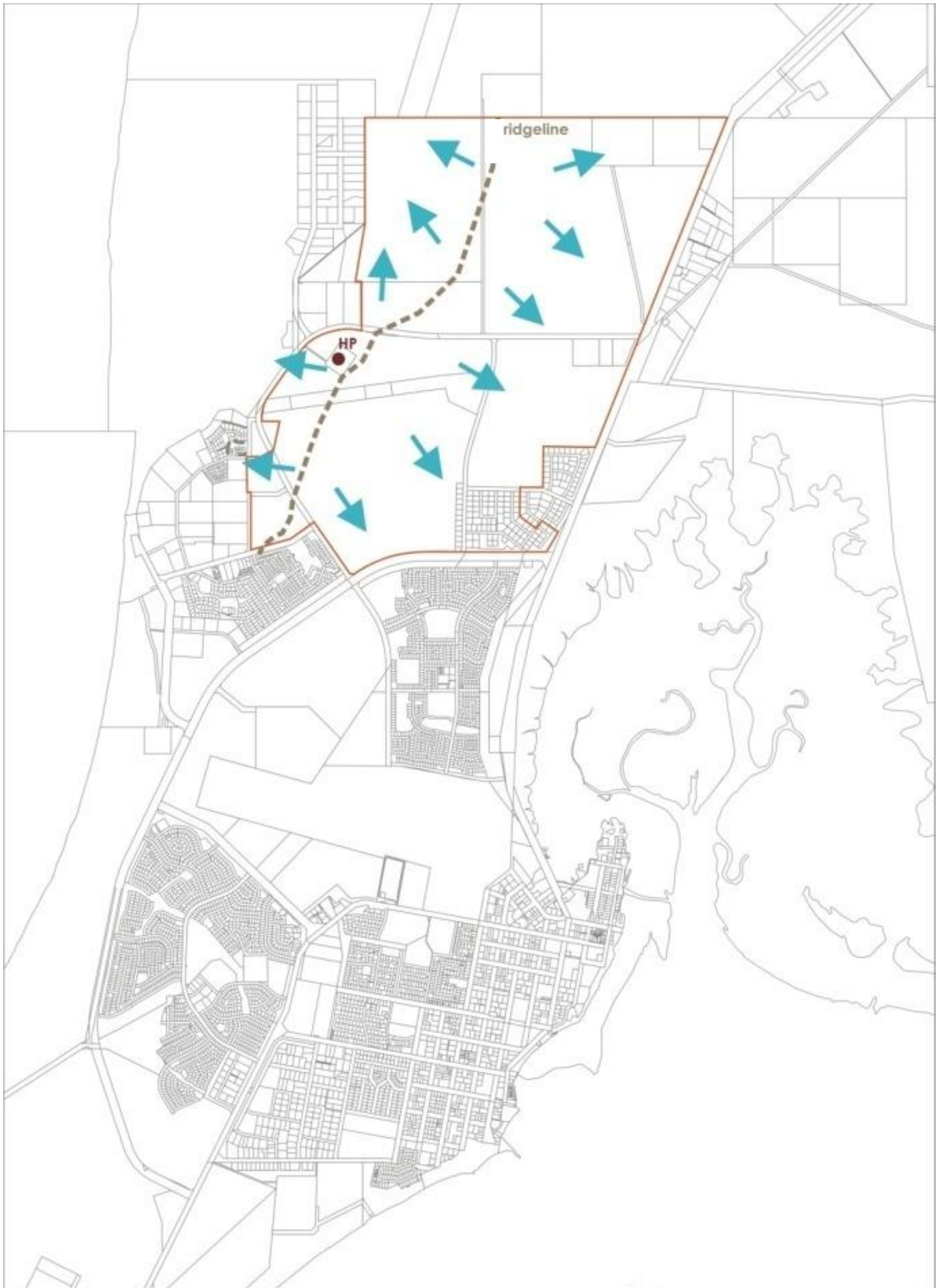
EXISTING DRAINAGE – BROOME NORTH SITE Drawn by UDLA, 2009 (using information from Broome Shire, Roberts Day and SKM)
