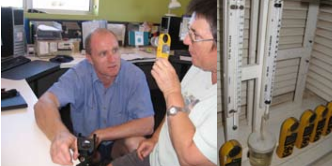
Bureau of Meteorology staff calibrating units for temperature, humidity and dew point.
