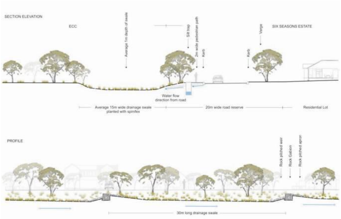
INITIAL DRAINAGE CONCEPTS Drawing by UDLA
