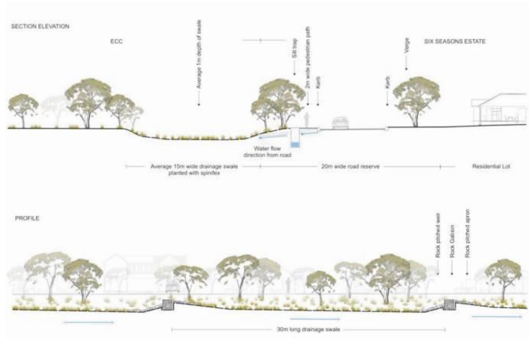
INITIAL DRAINAGE CONCEPTS Drawing by UDLA
