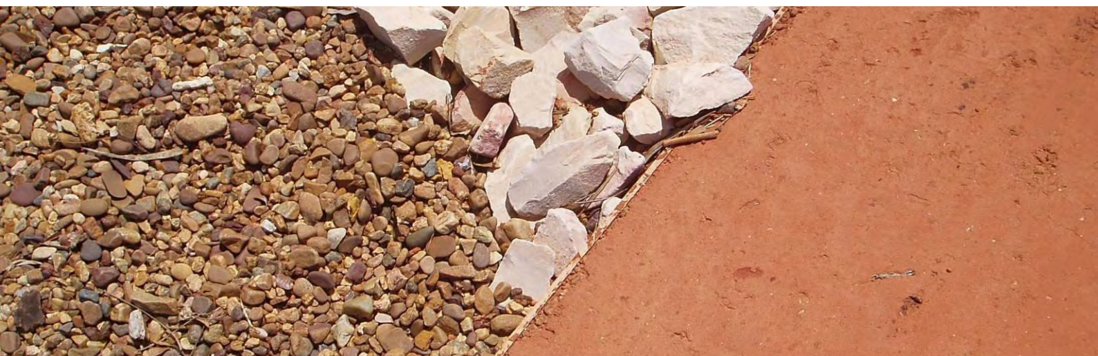
LOCAL MATERIALS – CEMENT STABILISED AND COMPACTED PINDAN PATH OVER PAGE CLEARED INFORMAL PINDAN TRACK Photos courtesy of UDLA
