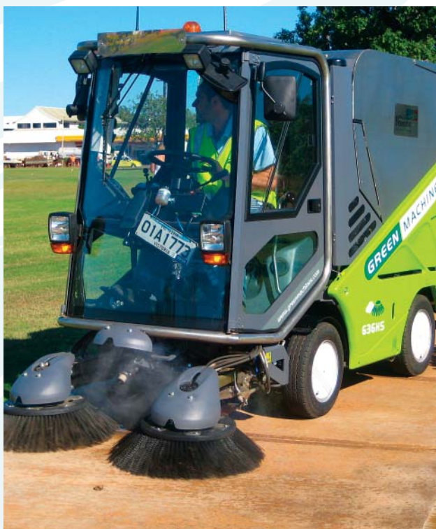
The new compact sweeper is designed to clean up leaves, broken glass, litter and dirt primarily on footpaths and car parks.
