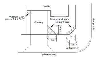
\*Fence in hashed area to be either less than 750mm in height or 80% visually permeable (i.e. pool fencing).
